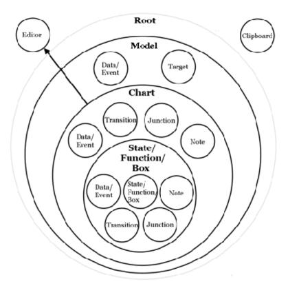
Rules of containment define the Stateflow hierarchy and the Stateflow API object hierarchy. For example, charts can contain states but states cannot contain charts. The hierarchy of Stateflow objects appears in the section "Stateflow Hierarchy of Objects" in the Stateflow and Stateflow® Coder™ User's Guide. The Stateflow API hierarchy consists of these layers of containment:
